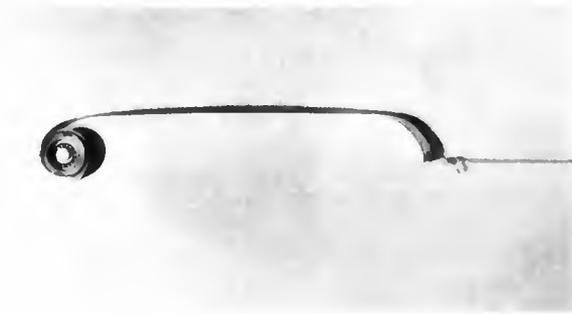
Fig. 8. Special Coil Spring with Constant Reaction
