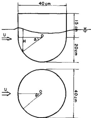
Fig. 6. Circular Cylindrical Type Buoy with Hemispherical Bottom
