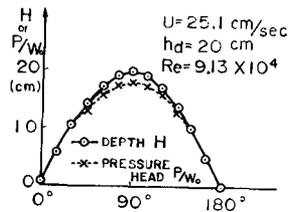
Fig. 7. Pressure Distribution on the Hemispherical Bottom
