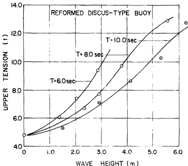
Fig. 15. Relationships between the Upper Tensions, Wave Heights and Wave Periods
