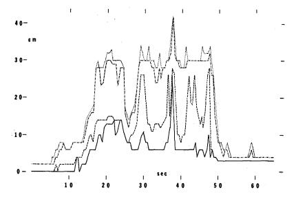
The average time between the sand fountains on the flood tide at the upper beachface is 1.7 minutes when the still water level is 0-30 cm below the station and 2.6 minutes when it is 0-30 cm above it. During the same tidal stages on the ebb tide, the average is 3.3 and 5.0 minutes respectively. Plotting the actual times between occurences (Figure 6) show that only two small peaks stand
