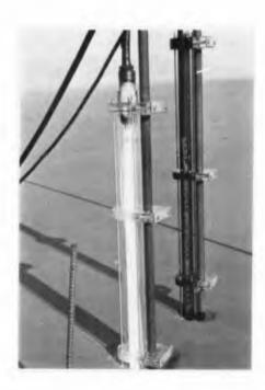
Figure 1. The almometer emplaced on the beach. The device consists of two acrylic cylinders; in one is a flourescent lamp in the other, 64 photo-electric cells.
