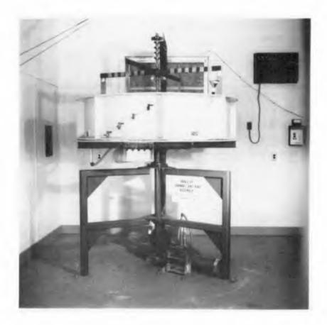
Fig. 1 Annular Channel and Ring Assembly.
