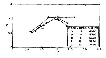
Fig. 9 Examples of Variation of  $\sigma_2$  with  $\tau_b^{\bigstar}$  for Kaolinite in Distilled Water.
