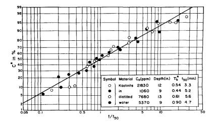
Fig. 8 Fraction of Depositable Suspended Concentration, C\*, versus Normalized Time  $t/t_{50}$  for Kaolinite in Distilled Water.
