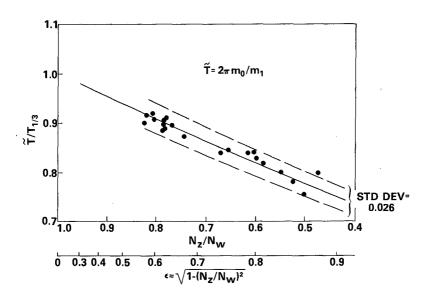
Figure 8. Spectral estimates of wave period
