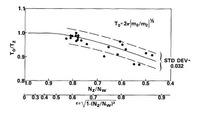
Figure 9. Spectral estimates of wave period
