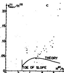
Fig. 9 Maximum relative skewness for waves with  $T = 1/6$  s
