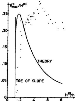
Fig. 6 Max. relative skewness  $T = 1/3$  s,  $H_0/L_0 = .0019$
