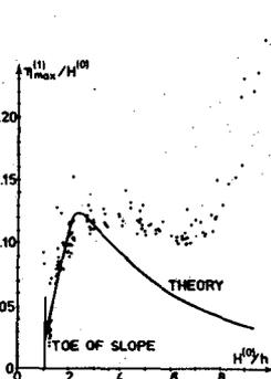
Fig. 8 Max. relative skewness  $T = 1/5$  s,  $H_0/L_0 = .0060$
