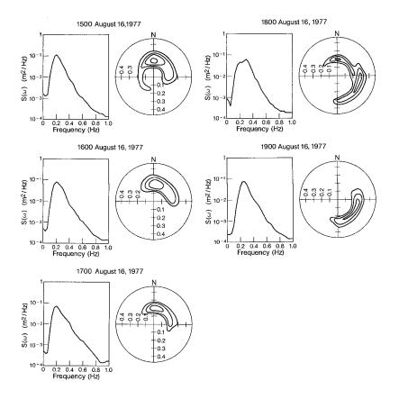
Fig. 10. Single and directional spectra during an episode with changing wind direction, August 16, 1977.
