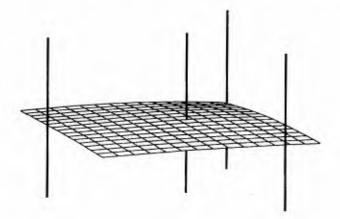
Fig. 2. An example of a fitted wave surface. The wave staffs are 6-m long.
