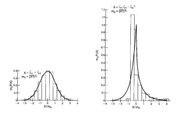
Fig. 6. Typical histograms of the distribution of mean and total curvatures. The non-normal distribution curve represents Longuet-Higgins' theory.
