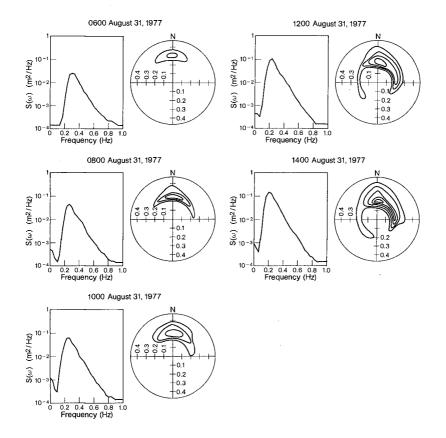
Fig. 9. Single and directional spectra during an episode with constant wind direction, August 31, 1977.
