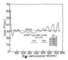
Fig. 9 Load-deformation curves of a one-eighth scale bow model of 4,000 G.T.
