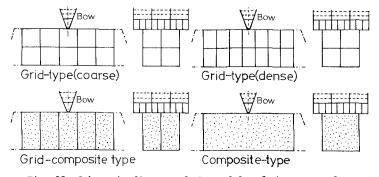
Fig. 13 Schematic diagram of the models of the proposed buffer devices  $% \left( {{{\rm{D}}_{{\rm{D}}}} \right)$
