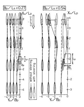
Fig. 3 Examples of the calculated ship trajectories ( $v_c/v_s = 0.75$ )
