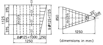
Fig. 7 One-fourth scale bow model of 500 G.T. ship
