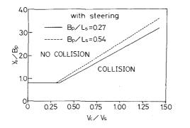
Fig. 5 The minimum required distance of the ship course from the pier center
