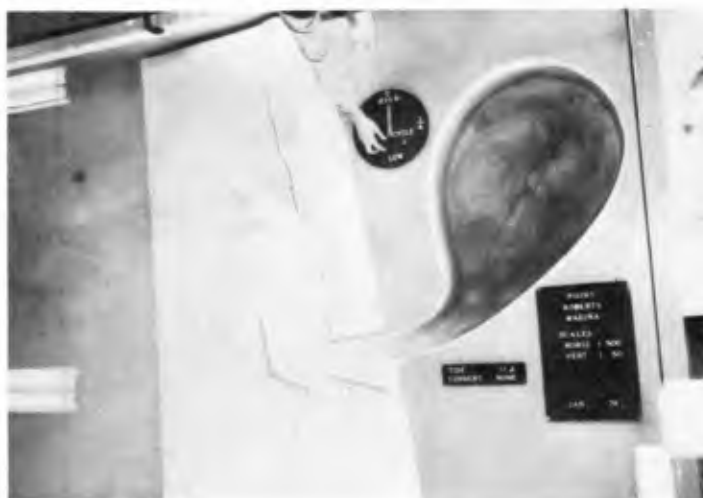
FIGURE 7B DISTRIBUTION OF DYE IN BOAT BASIN AT END OF FLOOD TIDE
