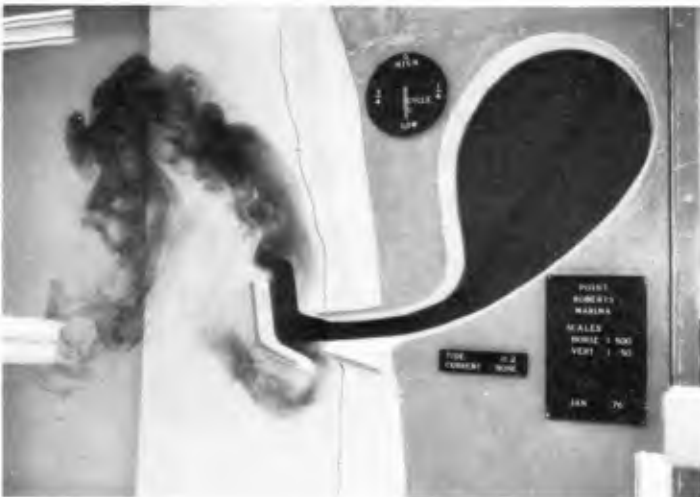
FIGURE 8B DISTRIBUTION OF DYE AT END OF EBB TIDE ( NO LONGSHORE CURRENT)
