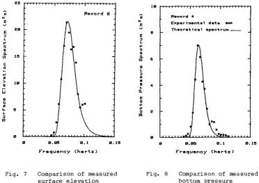
surface elevation spectrum with modified Wallops spectrum bottom pressure spectrum with modified Wallops type spectrum
