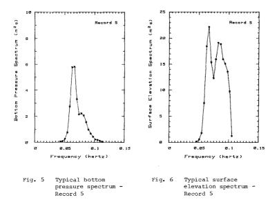
The period of the swell peaks ranged from 14.2 to 15.3 s, and estimated values of  $H_{\rm g}$  ranged from 2.1 to 3.1 m. Wave record 5 is typical and Figs. 5 and 6 represent respectively bottom pressure and surface elevation spectra for this record; in both representations swell and wind-sea peaks may be identified.
