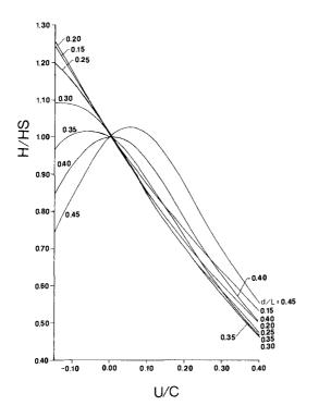
Fig. 10. The wave height change by Stokes (new) third order wave theory for  $\rm H_S/L_S=0.03$
