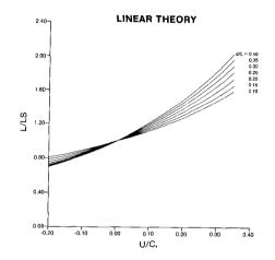
Fig. 2. Wave length change computed by linear wave theory (L/L\_S versus U/C)
