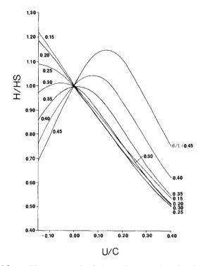
Fig. 11. The wave height change by Stokes (new) third order wave theory for  $H_S/L_S=0.05$
