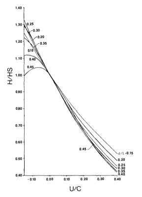
Fig. 9. The wave height change by Stokes (new) third-order wave theory for  $\rm H_S/L_S=0.01$
