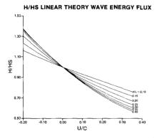
Fig. 4. The wave height change computed by linear wave theory
