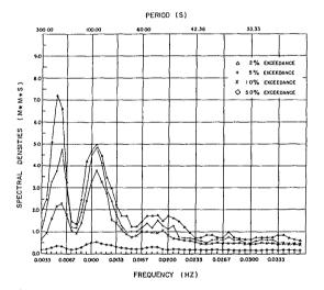
Figure 6 Spectral density exceedances for September 1981 at the entrance of the harbour
