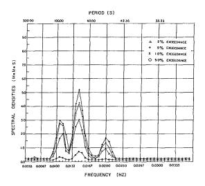
Figure 7 Spectral density exceedances for September 1981 inside the harbour PERNOD (S)
