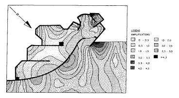
Figure 18 Maximum amplification for a period of 60,0 s
