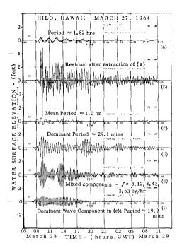
FIG. 9 - NUMERICALLY FILTERED AND PLOTTED WAVE-FORMS OF COM-PONENTS OF THE ALASKAN TSUNAMI AT HILO, HAWAII, MARCH, 1964
