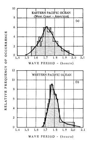
FIG. 14 - HISTOGRAMS OF WAVE PERIODS FOR "PRIMARY" LONG WAVE COMPONENT OF MARCH, 1964, ALASKAN TSUNAMI: (a) EASTERN PACIFIC OCEAN; (b) WESTERN PACIFIC OCEAN; (based on first three waves in Figs. 11 and 12)
