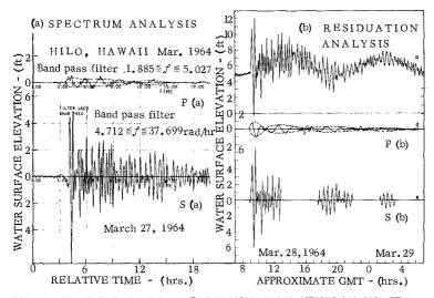
FIG. 7 - WAVE FORMS OF LOW-FREQUENCY COMPONENTS (P) AND SEC-ONDARY COMPONENTS (S) IN MARIGRAM OF MAR. 28, 1964, FOR HILO, HAWAII. Spectrum analyses (a) used parameters F (Table I); Residuation analyses (b) are graphical.
