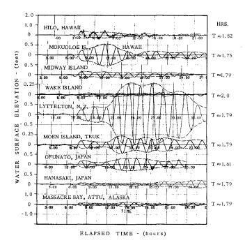
FIG. 12 - COMPUTER-PLOTTED WAVE-FORMS OF LONG-PERIOD COMPON-ENT (AVERAGE PERIOD 1.77 HRS) OF THE MARCH, 1964, ALASKAN TSUNAMI, NUMERICALLY DETERMINED FROM MARIGRAMS OF PAC-IFIC OCEAN TIDE-STATIONS: (ordinate scales not uniform; envelopes hand-drawn).
