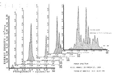
FIG.8 - WAVE-ENERGY SPECTRA FROM DATA S(a) IN FIG.7, AS FILTER-ED THROUGH BAND-PASS FILTERS (a) TO (f), HILO, HAWAII.
