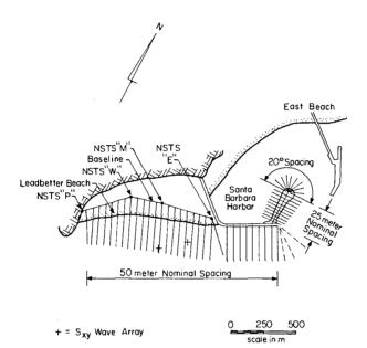
Figure 3 Plan of Sediment Impoundment Study and Location of Directional Wave Gages
