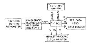
Figure 4 Block Diagram of OSI's Data Acquisition System
