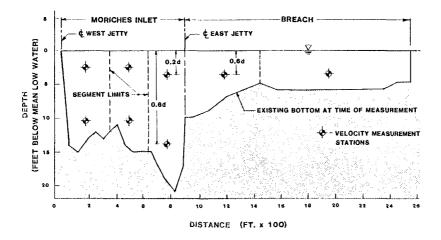
Figure 12 - Current Profiling Station Locations
