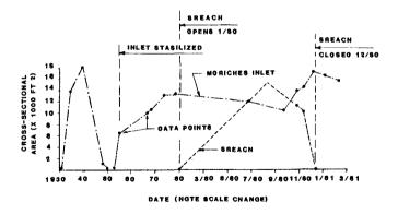
Figure 14 - Inlet/Breach Cross-Sectional Area Changes
