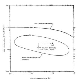
Figure 3. Least squares estimated bedload and suspended load efficiency factors,  $\epsilon_{\rm B}$  and  $\epsilon_{\rm S}$ .
