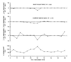
Figure 4. Comparison between predicted beach volume changes (a, b) and measured beach volume changes (c). The volume changes shown in (a) were predicted from Equation 4 using the measured wave heights (d), while the volume changes shown in (b) were predicted from Equation 1.
