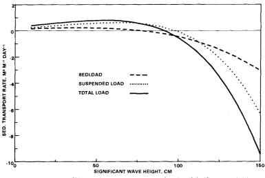
Figure 5. Predicted on-offshore sediment transport rate as a function of significant wave height. The individual contributions of the bedload and suspended load transports to the total transport are shown by the dashed and dotted lines, respectively. The point of neutral transport (equilibrium) occurs at a significant wave height of 90 cm.
