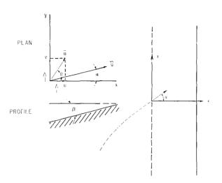
Figure 1. Schematic diagram showing the position of the beach (solid line), the breakpoint (dashed line), the wave angle  $\alpha$  and the oscillatory and steady water velocities  $\widetilde{u}$  and u (from Bailard and Inman, 1980, with permission).
