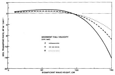
Figure 6. Predicted total load on-offshore sediment transport rate as function of significant wave height and sediment fall velocity. Greater rates of transport are found for smaller sized sediments.
