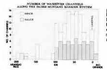
Figure 10. Locations of hurricane channels cut across Padre-Mustang Barrier System by Hurricane Allen. Major channels are those cut below mean sea level, minor channels are less deep.
