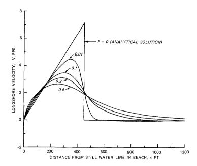
Figure 6. Plane Beach: Effect of mixing parameter P on the numerical solution (set-up is neglected)
