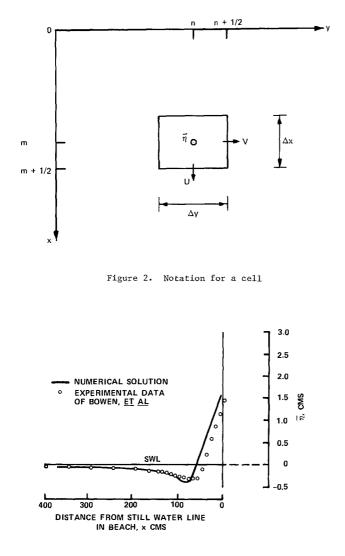
Figure 3. Comparison of the numerical solution for set-up with experimental data
