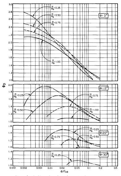
Figure 5. Nonlinear Drag Force Correction Factor.
