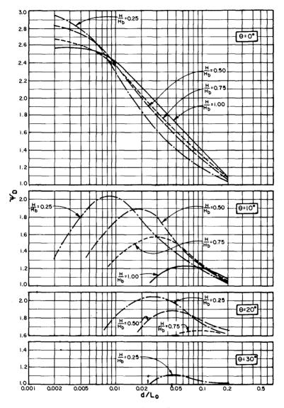
Figure 9. Nonlinear Drag Moment Correction Factor.
