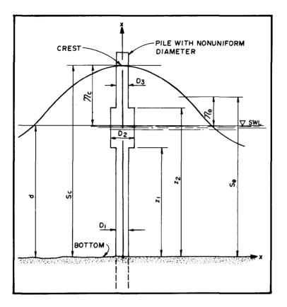
Figure 1. Definition Sketch for a Pile with Three Diameters.
