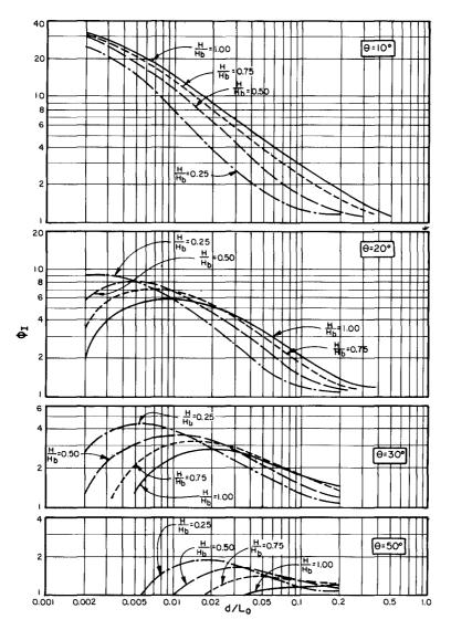
Figure 6. Nonlinear Inertial Force Correction Factor.
