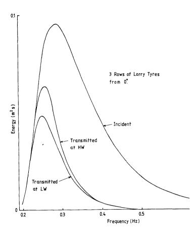
Fig. 4 - Breakwater Performance for 3 rows of lorry tyres with waves from  $\text{O}^{\text{O}}$
