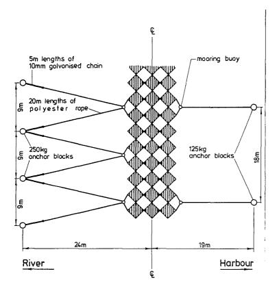
Fig. 6 - Mooring arrangement for floating tyre breakwater at Port Edgar
