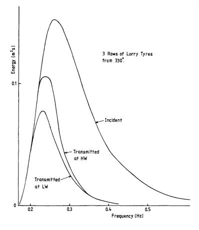
Fig. 3 - Breakwater Performance for 3 rows of lorry tyres with waves from  $330^{\rm O}$
