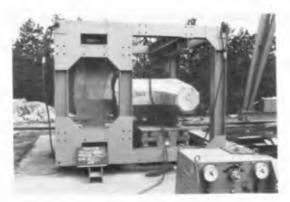
Photograph 3: The breakage of Dolos (Static loac test)
