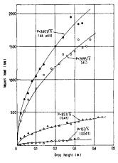
Figure14 Relationship between impact load and drop height
