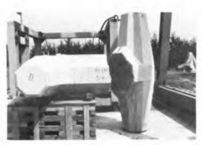
Photograph 5: The breakage of Dolos (Drop test)
