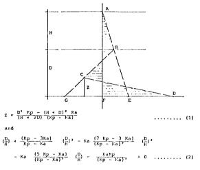
The following values of 'D' have been calculated compatible with the probable values of  $K_{\rm p}$  and  $K_{\rm a}.$
