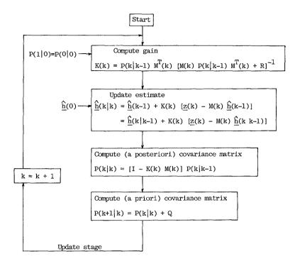
Fig. 6.-- Algorithm of Kalman Filtering
