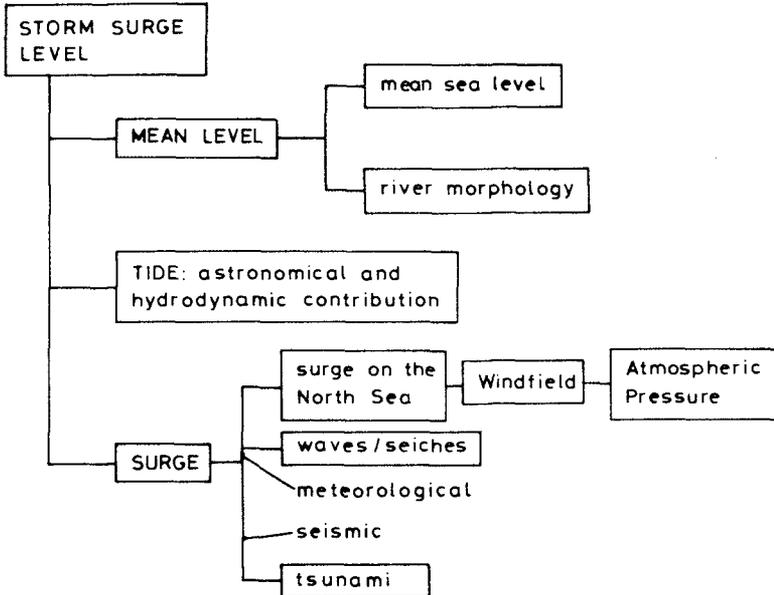
Fig.1: Components of storm surge level
