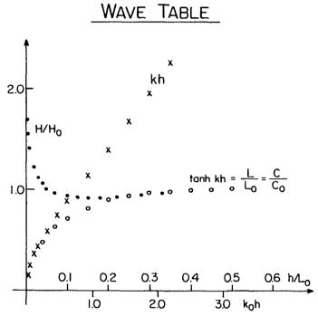
Figure 3: A wave table provides discrete values of commonly used wave parameters in terms of  $k_0h$  or  $h/L_0. \\$
