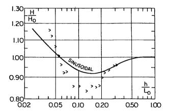
Figure 1: Measured values of the shoaling coefficient  $\rm H/H_{0}$  compared to linear theory (After Brink Kjaer and Jonsson 1973). The error is of the order 10 percent.
