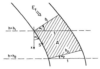
Figure 6: Definition diagram for wave height predictions over straight parallel bottom contours.
