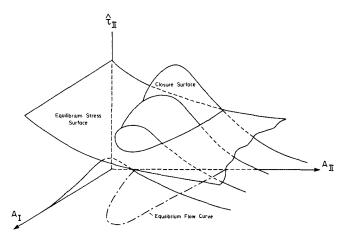
Fig. 2 Closure surface and equilibrium stress surface
