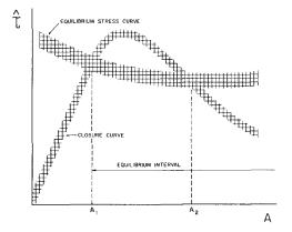
Fig. 1 Closure curve and equilibrium stress curve
