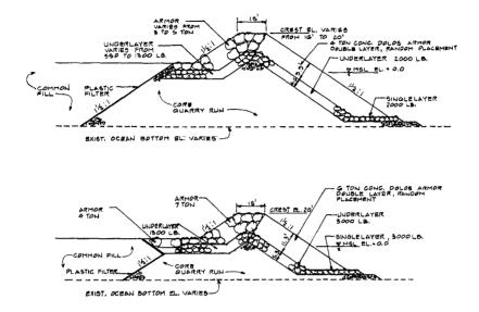
FIG.2 TYPICAL DOLOS ARMOR PROTECTIVE STRUCTURE SECTIONS (Not To Scale)
