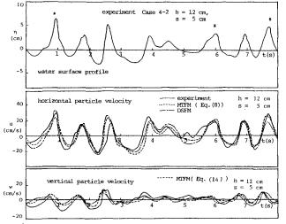
Fig.ll Time profile of water particle velocities for irregular wave (Case 4-2, h=l2cm and s=5cm).
