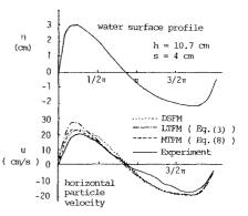
Fig.1 Comparison between measurement and calculations (Regular wave; experimental and DSFM's values are from Nadaoka et a1.4).
