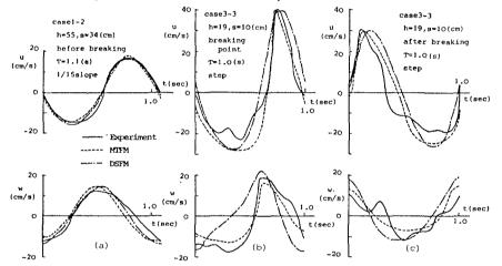
Fig.9 Comparison of time profiles of water particle velocities between calculations and experiments (for regular waves)
