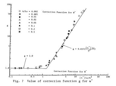
According to Figs. 6 and 7, the correction function g can be approximated by
