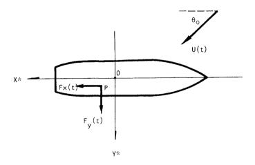
Fig. 4 The definition of wind direction  $\theta_{\Omega}$
