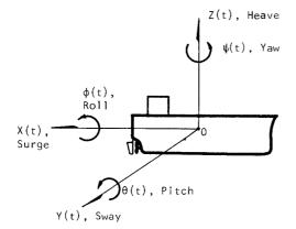
Fig. 2 The definition of six ship motions
