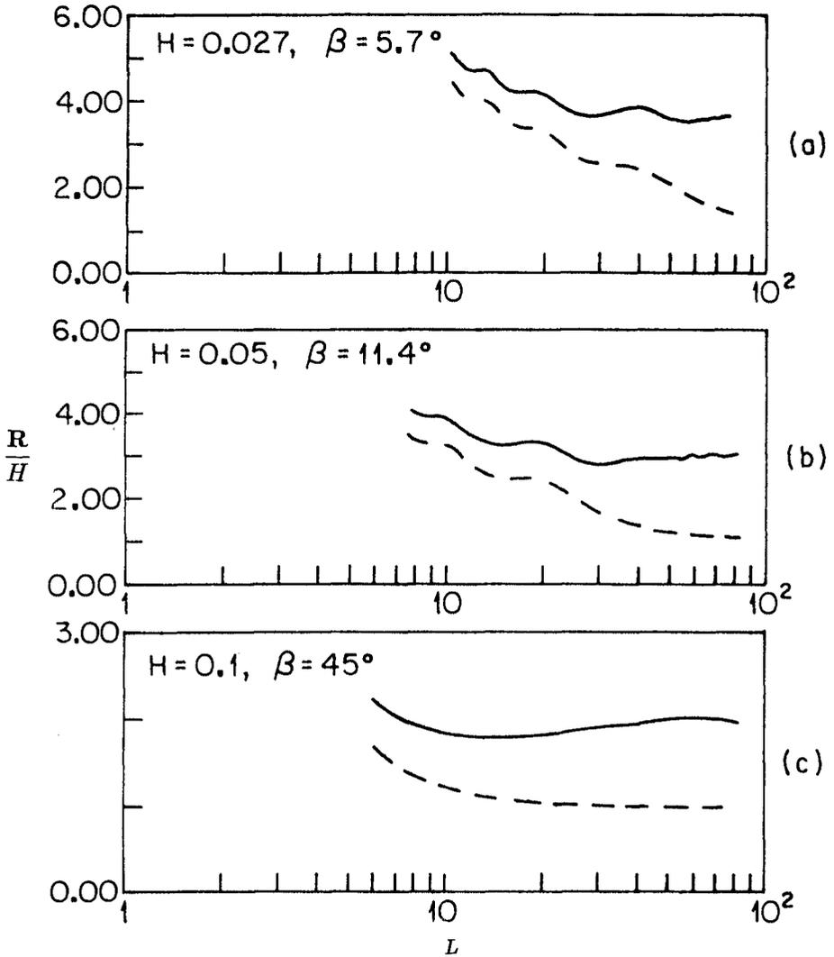
**Figure 3** The maximum relative runup of sinusoidal waves (dashed lines) and the maximum relative runup of cnoidal waves (solid lines) with the same height  $H$  up three sloping beaches as a function of the dimensionless wavelength. (a)  $H = 0.027, \beta = 5.7^\circ$ ; (b)  $H = 0.05, \beta = 11.3^\circ$ ; (c)  $H = 0.1, \beta = 45^\circ$ . Nonbreaking waves.
