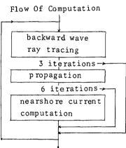
Fig. 4 Schematic diagram of computation flow.
