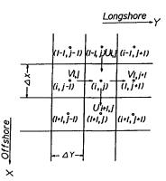
Fig. 3 Configurations of variables in finite difference model.
