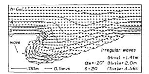
Fig. 14 Spatial distribution of nearshore current patterns on a curved bay computed by the numerical models with regular and irregular wave theories.
