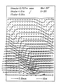
Fig. 11 Nearshore current patterns on asymmetrical concave topography.
