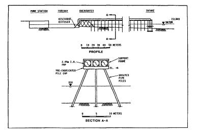
Figure 4. Pump/siphon water intake on trestle.
