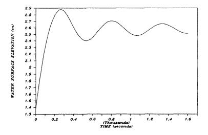
Figure 7. Surge analysis for pump shut-down conditions.
