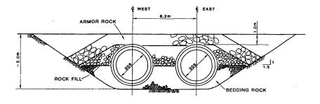
Figure 5. Buried concrete pipe design with backfill.
