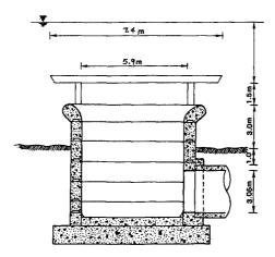
Figure 3. Offshore submerged intake riser.
