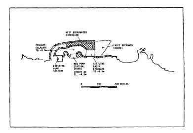
Figure 2. Onshore intake with parallel breakwater.
