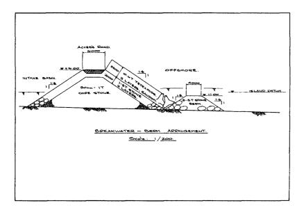
Figure 6. Breakwater cross-section showing berm and tetrapods.
