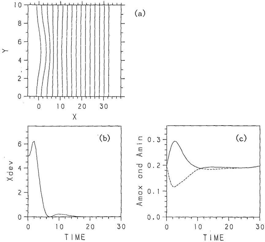
Fig. 4 (a) The top-view of the crest-line for  $0 \leq t \leq 30$ . (b)  $X_{\text{dev}}$ , i.e., the deviation of the crest-line from a straight line. (c) The evolution of the maximum and the minimum waveheight along the crest-line ( $a_0 = 0.2$ ,  $L_y = 10$  and  $\epsilon = 1$ )
