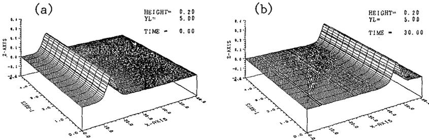
Fig. 2 Wave-form when the solitary wave is not bent initially.
