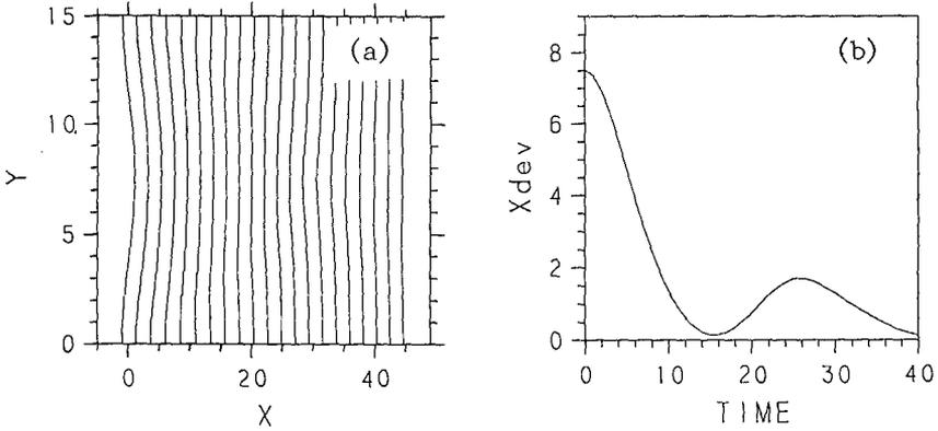
Fig. 6 (a) The top-view of the crest-line for  $0 \leq t \leq 40$ . (b)  $X_{dev}$ , i.e., the deviation of the crest-line from a straight line. ( $a_0 = 0.2$ ,  $L_y = 15$ ,  $\epsilon = 1$  and the energy conservation eq.(8) is assumed.)
