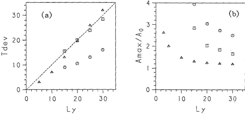
Fig. 7 (a)  $L_y$ -dependence of the characteristic time-scale (b)  $L_y$ -dependence of the maximum waveheight that appears during the transient motion.  $\circ$  : model with mass conservation,  $\square$  : model with energy conservation,  $\triangle$  : SMCE.
