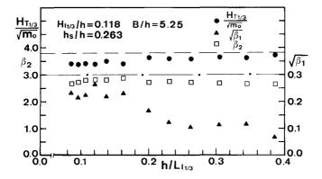
Figure 10 Relationship between the spectrum and the significant wave height and nonlinearity parameters for transmitted-wave trains.
