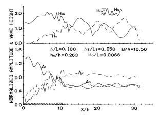
Figure 3 Spatial distribution of the amplitude of harmonic components for the finite plate (B/L = 10.50, h/L = 0.100).
