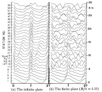
Figure 1 Wave profile transformation along the wave tank  $(h/L = 0.100, H_I/L = 0.0066)$ .
