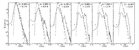
Figure 8 Transformation of the spectral shape of random waves measured along the tank  $(h/L_{I_{1/3}} = 0.105, H_{I_{1/3}}/h = 0.118); ---$  target spectrum, ••••• incident wave, transmitted wave.
