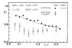
Figure 13 The average, maximum and minimum wave transmission coefficient versus relative water depth.
