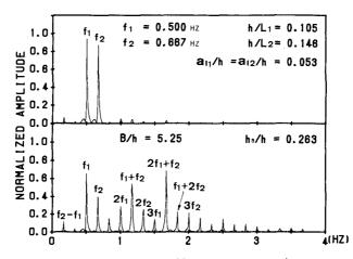
Figure 5 Amplitude of spectra of the incident wave of two primary components(upper) and the transmitted wave (lower).
