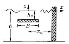
Figure 11 Schematical description of a submerged horizontal plate and vertical permeable wall.
