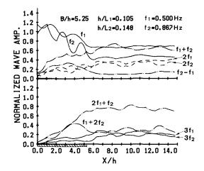
Figure 6 Spatial distribution of harmonic component amplitudes, measured along the tank, for two primary waves.
