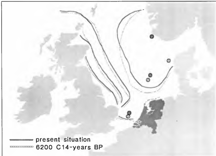
Figure 5 Iso-amplitude lines and amphidromic points corresponding to the semi-diurnal tide (after Franken, 1987).
