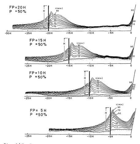
Fig. 8(d) The time evolution of the sand accumulation around fence placed in front of an embankment (P=50%).
