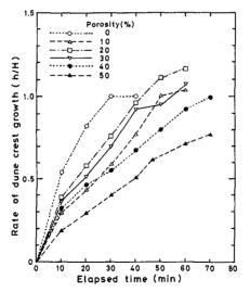
Fig. 5 Dune crest growth rate with elapsed time for different fence porosity
