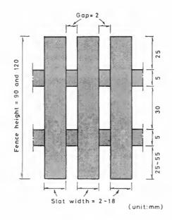
Fig. 1 Dimensions of the model fence.
