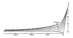
Fig. 7 Sand accumulation in front of an embankment.
