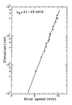
Fig. 3 Vertical distribution of wind speed on a fixed bed.
