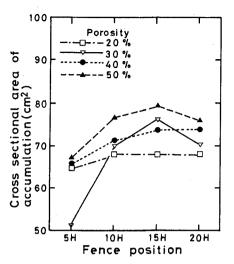
Fig. 9 Cross-sectional area of accumulated sand as a function of fence porosity and position.
