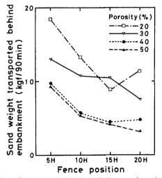
Fig. 10 Sand weight transported beyond embankment as a function of fence porosity and position.
