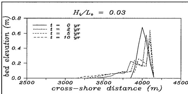
Figure 2 Cross-shore spreading of a triangular beach fill for a high steepness wave climate (SWL at 4000 m)
