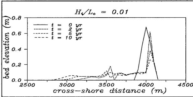
Figure 1 Cross-shore spreading of a triangular beach fill for a low steepness wave climate (SWL at 4000 m)
