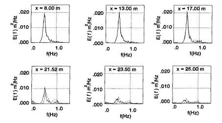
Figure 3: Observed (solid line) and computed (dashed line) frequency spectra in Schelde flume experiment at 6 locations.
