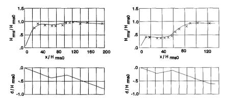
Figure 1: Observed (crosses) and computed (solid line) variation of the root mean square wave height  $H_{rms}$  and water depth d, normalized with the deep water rms wave height  $H_{rms0}$ , for the cases 13 (left panel) and 15 (right panel) of Battjes and Janssen (1978).
