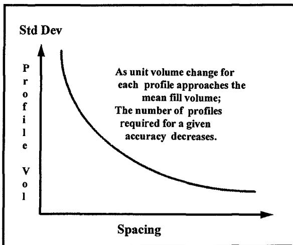
**FIGURE 6.** Conceptual model of the relationship of profile volume variance to profile spacing. For projects where the variance of profiles is high, more closely spaced are required to yield the "true" volume change.
