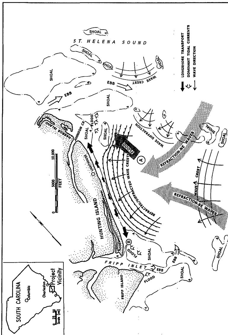
**FIGURE 1.** General model of coastal processes producing refraction and diffraction around shoals and sand transport away from the center of Hunting Island. Shoals are defined by the -6 ft (-1.8 m) mean low water contour as depicted on U.S. National Ocean Survey Chart No. 11513 (after CSE, 1990).
