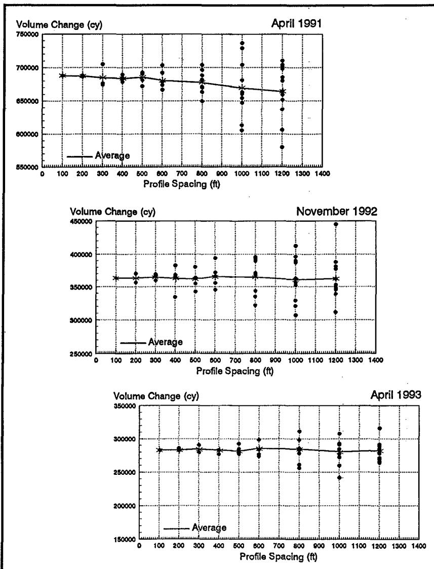
**FIGURE 7.** Computed sand volume changes since nourishment as a function of profile spacing for April 1991 (upper), November 1992 (middle), and April 1993 (lower) in the project area (stations 3+42 to 83+31). Averages are arithmetic and are not weighted for minor variations in profile spacing or for the fact that the ends of most profile pairs will not equal the nominal spacing, as explained in the text. After Kana and Andrassy (1993).
