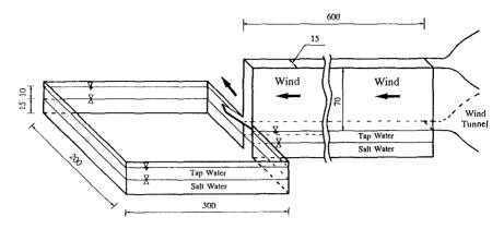
Figure 7. Experimental facility of two-layer stratified flow system with wind tunnel
