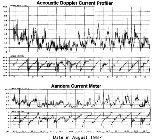
Figure 4. Currents measured by an ADCP and an Aandera current meter in Typhoons Betty and Cary.
