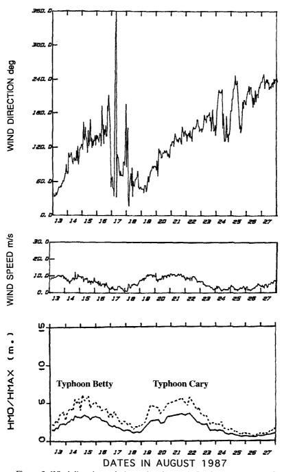
Figure 3. Wind direction, wind speed and wave in Typhoons Betty and Cary.
