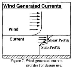
current near sea surface which should be associated with the design wind and wave could be very different depending on whether a shear or a slab current profile (Figure 7) is
