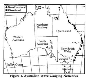
The wave data network in New South Wales presently consists of seven stations, one of which collects directional data (Figure 1). The oldest station in this network was installed in 1974; all stations have been operational since 1987. Datawell Waverider buoys are used at every station, and the data are transmitted to a shore station by radio.
