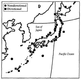
Figure 6. NOWPHAS and JMA Wave Measurement Stations
