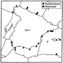
Figure 10. Spain's Coastal Wave Gauging Network
