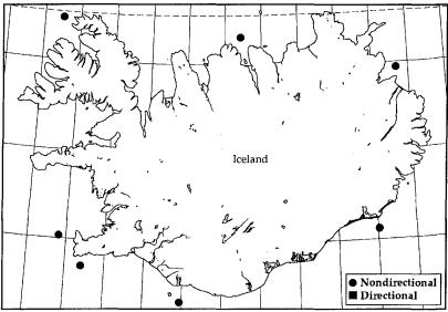
Figure 4. Icelandic Data Buoy Network
