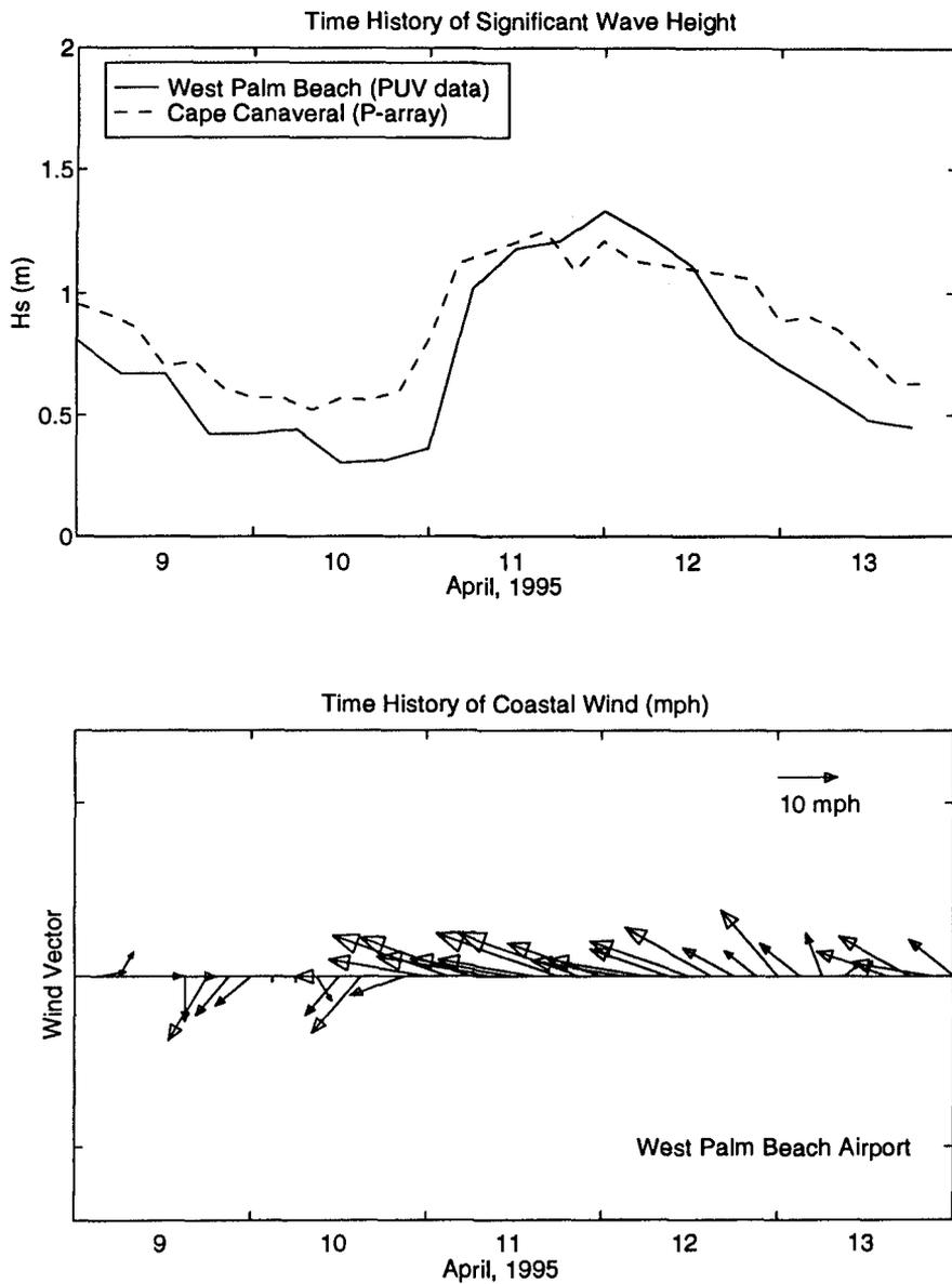
Figure 4: Measured significant wave heights and surface winds.
