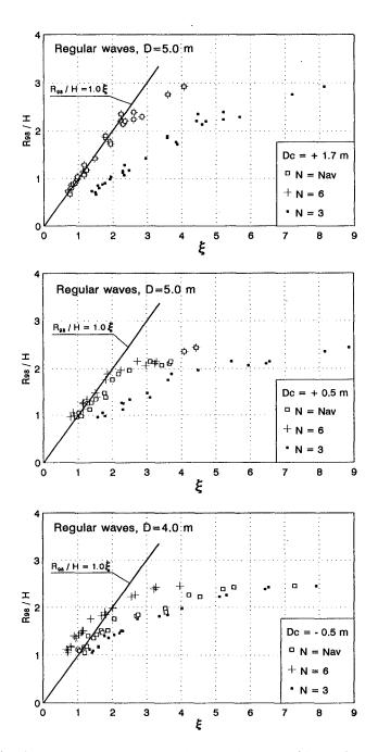
Fig. 4 :  $R_{98}$  / H versus breakerindex  $\xi$  for tests with regular waves
