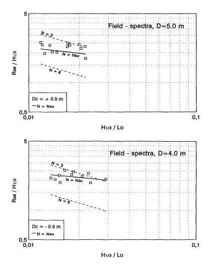
Fig. 8 :  $R_{98}$  /  $H_{1/3}$  versus steepness  $H_{1/3}$  / Lo for tests with field-spectra
