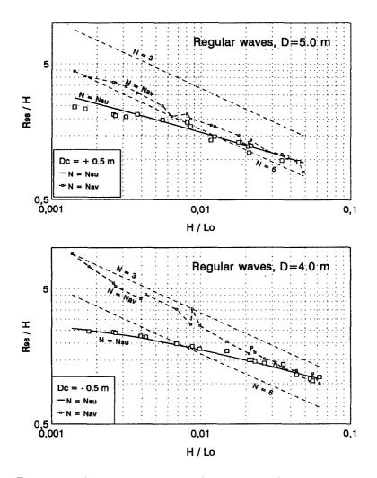
Fig. 5 :  $R_{98}$  / H versus steepness H / Lo for tests with regular waves
