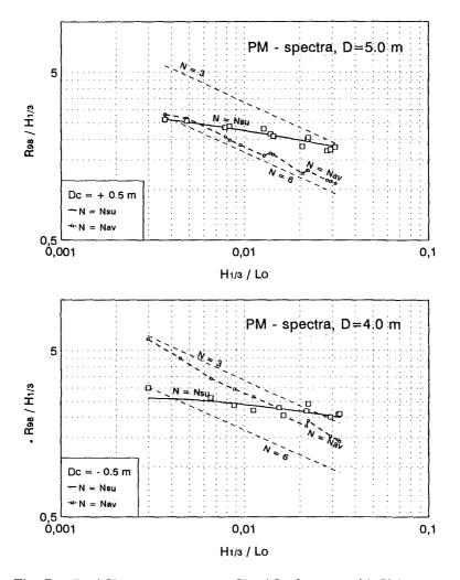
Fig. 7 :  $R_{98}$  /  $H_{1/3}$  versus steepness  $H_{1/3}$  / Lo for tests with PM-spectra
