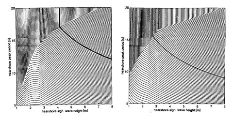
Fig. 8. Contours of run-up reliability function z as function of nearshore significant wave height and nearshore peak wave period for sea level 3.0 m (left) and 5.0 m (right) at Pettemer Zeewering (ref. de Valk 1996).
