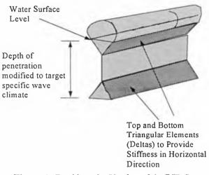
Figure 4. Double Delta Version of the RIB System
