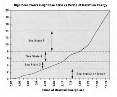
Figure 3. Relationship Between Sea State, Significant Wave Height and Period.
