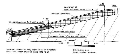
Figure 1 Example of a placed block revetment
