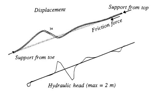
Figure 7 Hydraulic head difference (lower part) and corresponding displacement (upper part)
