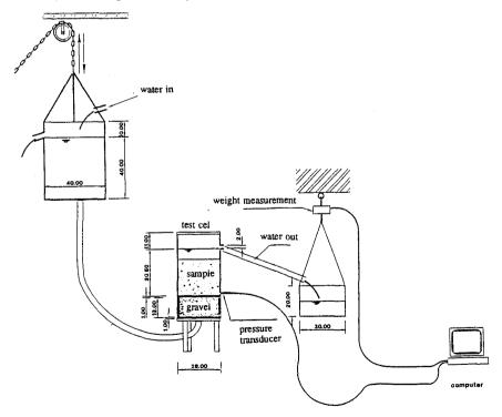
Figure 6 Set up for tests on sand-grain mixtures
