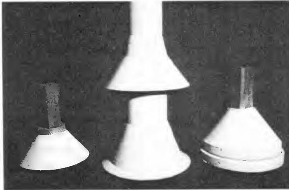
Figure 5 - 1:70 Scale Models of Bridge Piers
