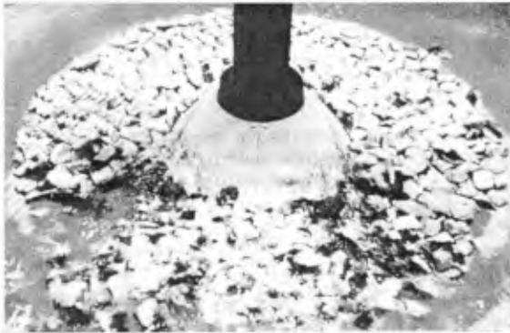
Figure 10 - Scour Protection Test at Shallow Water Approach Pier
