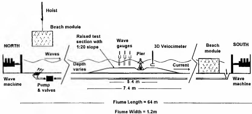
Figure 6 - Schematic Diagram of Test Flume
