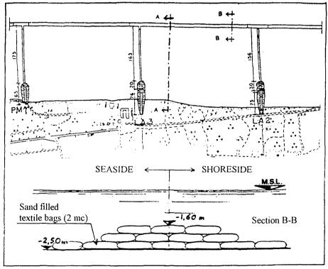
Fig. 2 - Protective system whit sandbags - New intervention.
