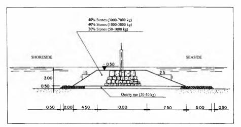
Fig. 6 - Submerged breakwater at Marina di Montemarciano (AN, Marche).
