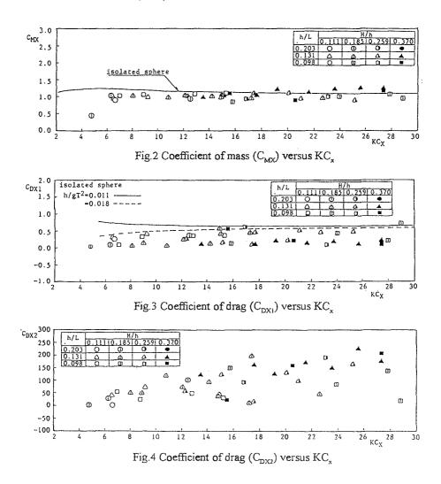
It is clear in Fig.2 that the value of  $C_{MX}$  is almost constant and independent of  $KC_x$ . Also, the values for isolated spheres and armor spheres are very similar. The value of  $C_{MX}$  has been estimated to be 0.96 ( $C_{AX}$  = -0.04) by taking the average over all computed values. This value has been used in the numerical model for comparison with the experiment.
