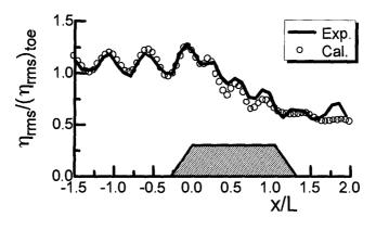
Fig.7 water level variation along the wave tank ( $h/gT^2 = 0.015$ , H/h = 0.11)
