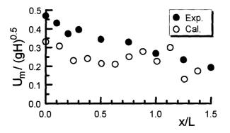
Fig.8a Maximum horizontal porewater velocity along the crown  $(h/gT^2 = 0.029, H/h = 0.11)$
