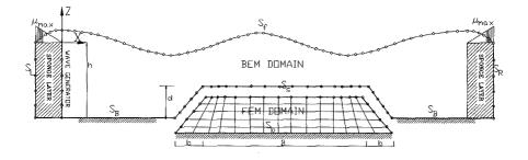
Fig.1 Wave tank for wave-submerged breakwater dynamic interaction
