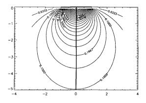
Figure 2: Infinite depth solution. Total impulse on deck (0,1) is  $\pi/4$ .
