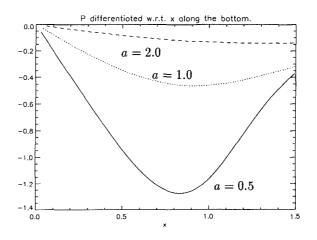
Figure 12:  $\frac{\partial P}{\partial x}$  along the bottom.
